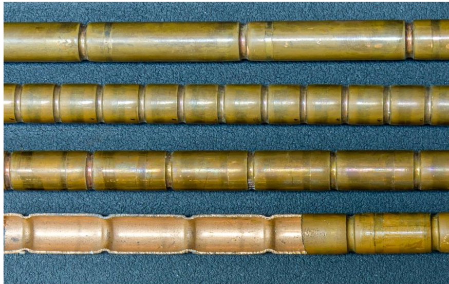
Figure 1. 1: Cylindrical tubes with repeated ring type grooves at different pitch ratios [8]
