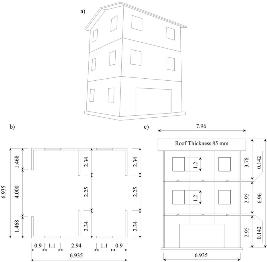
**Fig. 5** a) The three-story building of the SOFIE project configuration C b) first floor plan, c) south wall elevation (units in meters) (Ceccotti 2008)
