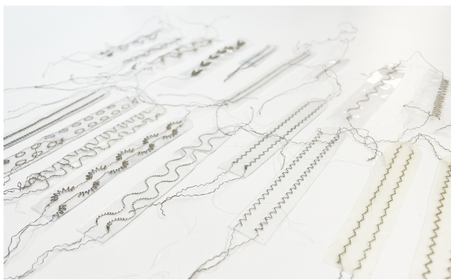
Figure 2: During the design process of the sewn tactful sensor we experimented with different stitching options and silicone types. The final prototypes were made with 1.5mm thick Smooth-On EcoFlex 00-20 platinum cure silicone. Some versions had SLIDE™ STD Liquid Surface Tension Diffuser added to provide a softer, less tacky sensation.
