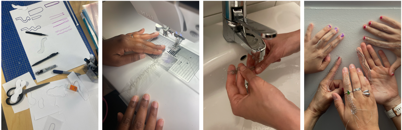
Figure 3: Fabrication process of the sewn sensor, from left to right: cutting out silicone shapes for the base of the sensor, sewing into a silicone shape ‘sandwiched’ between two PVA sheets, washing off the PVA sheets, final sensors adhered to the hand.
