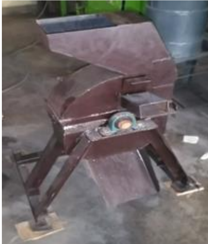
Figure 1: Biomass size reduction machine used for milling corncobs
