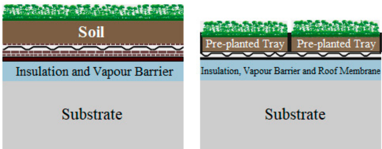
Figure 5. Green roof systems as intensive (left) and extensive (right) [57].
