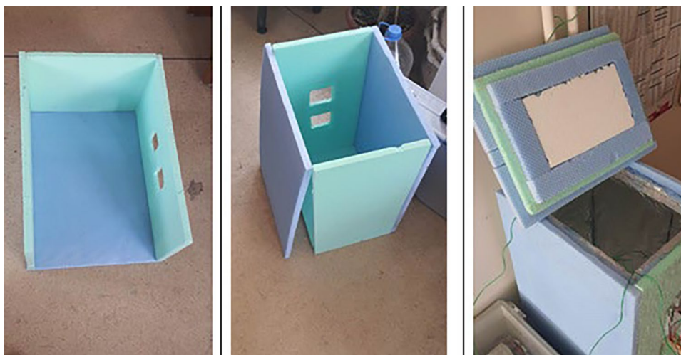
Fig. 4 Manufacturing of cooling cabinet
