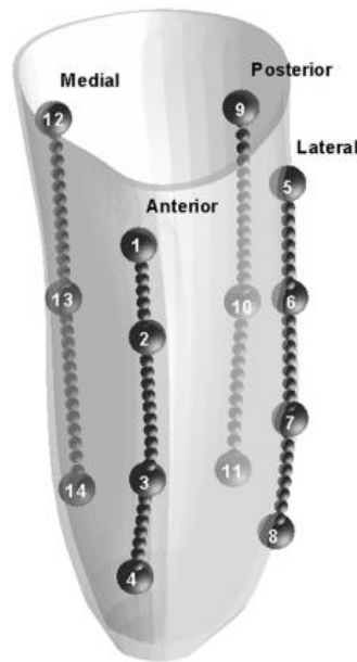
Figure 4: Locations of temperature data acquired experimentally (large spheres) and extracted from the numerical model (small spheres) of a residual limb (source Peery et al. 2006)
