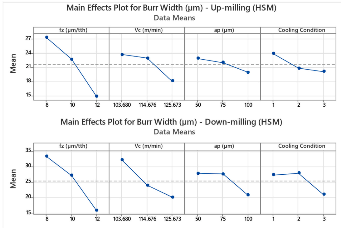
Fig. 15. Main effects plot illustrating the influence of process parameters on burr width ( \mu\text{m} ) – up-milling and down-milling (HSM).
