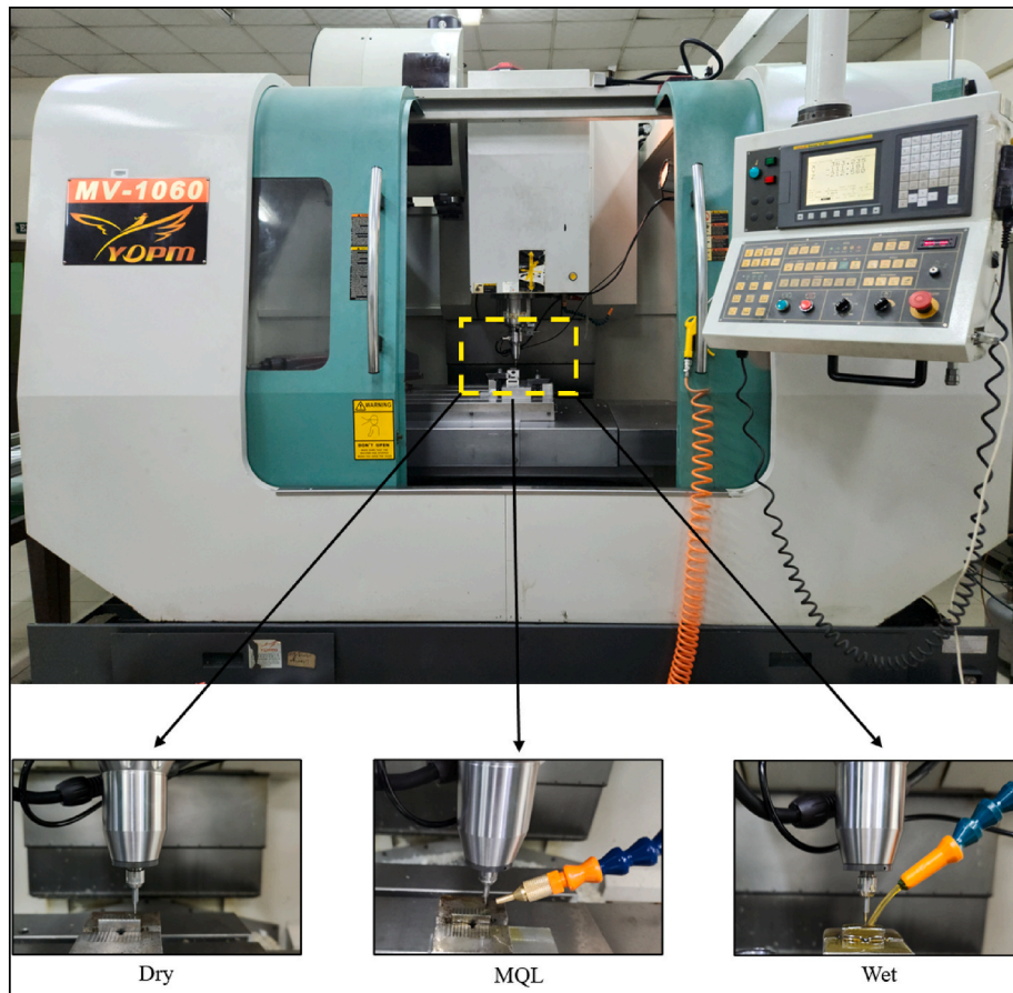
Fig. 3. Experimental setup illustrating machining under dry, MQL and wet cooling conditions.
