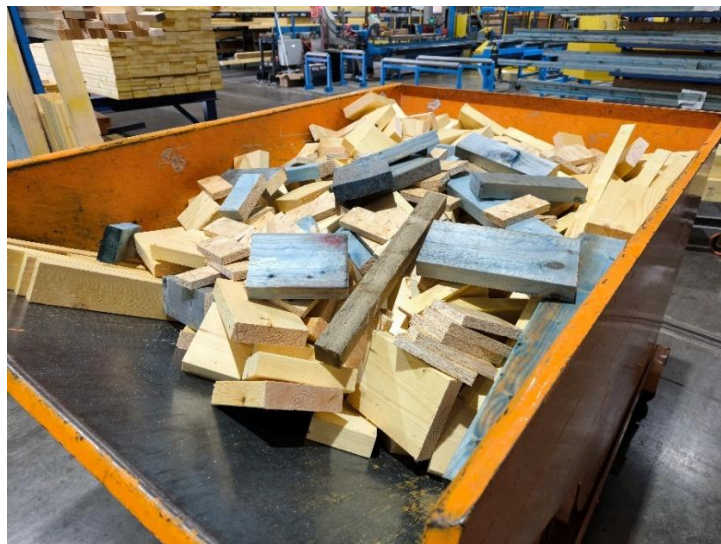
Figure 5.33: Various timber offcuts resulting from limited nesting
