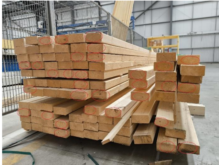
Figure 5.18: Cracked and uneven standard timber edges
