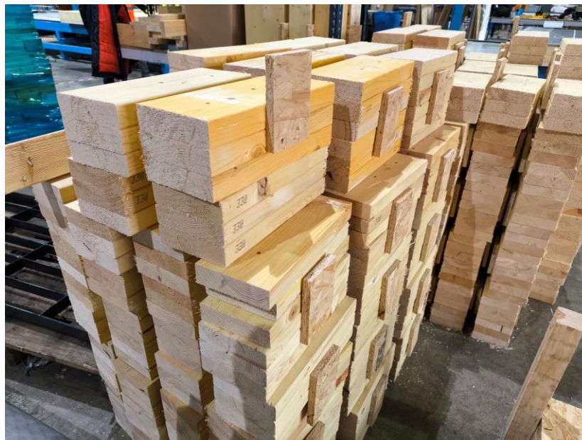
Figure 5.32: Timber offcuts being repurposed as transportation props
