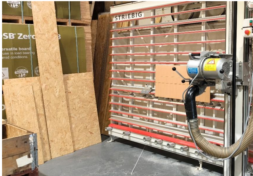
Figure 5.43: Length-side OSB offcut accumulation
