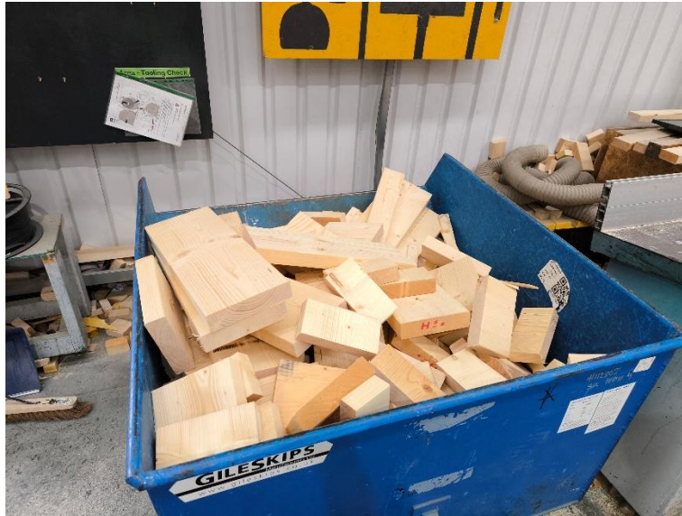
Figure 5.42: Various offcuts generated because of limited nesting practice
