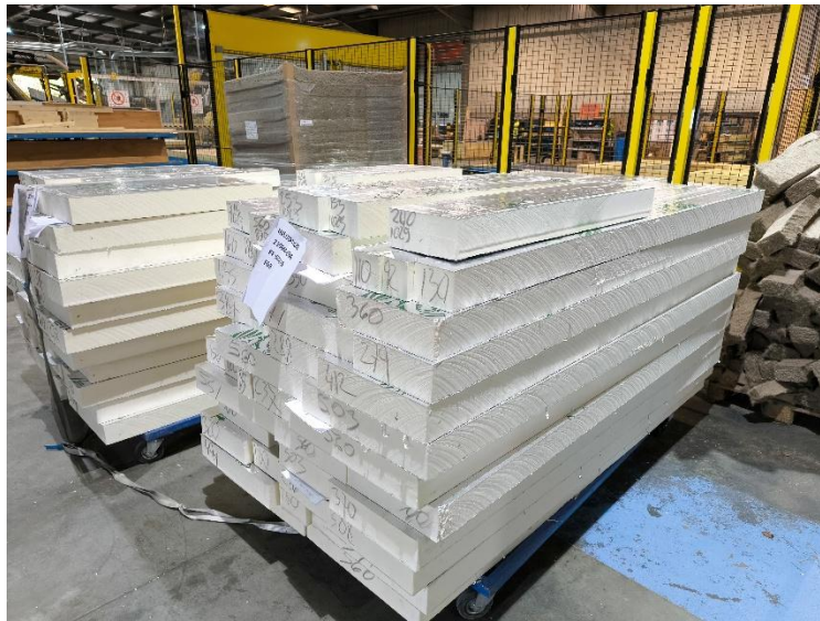
Figure 5.37: Rigid insulation cuts being prepared in required sizes
