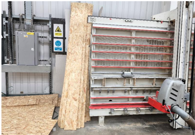
Figure 5.20: Width-side OSB offcuts being stored for future reuse
