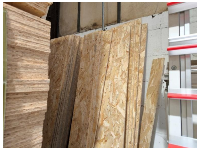
Figure 5.44: Width-side OSB offcut accumulation
