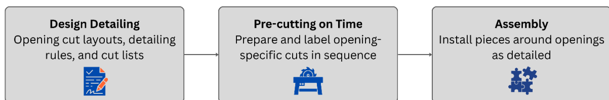
Figure 8.2: Adopting cut planning around openings
