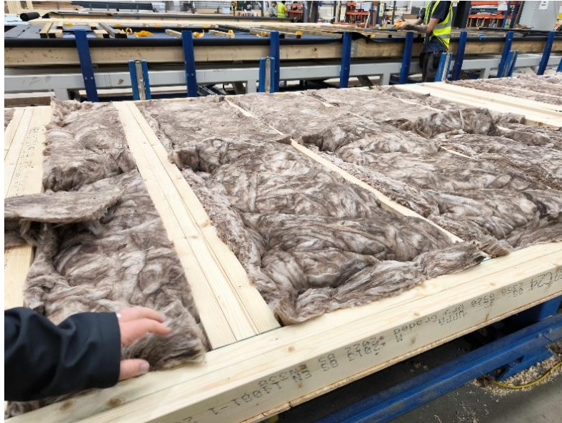
Figure 5.46: Overstuffing practice of rockwool insulation
