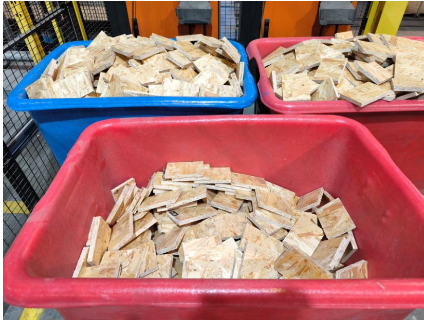
Figure 5.35: OSB offcuts being repurposed as transportation props
