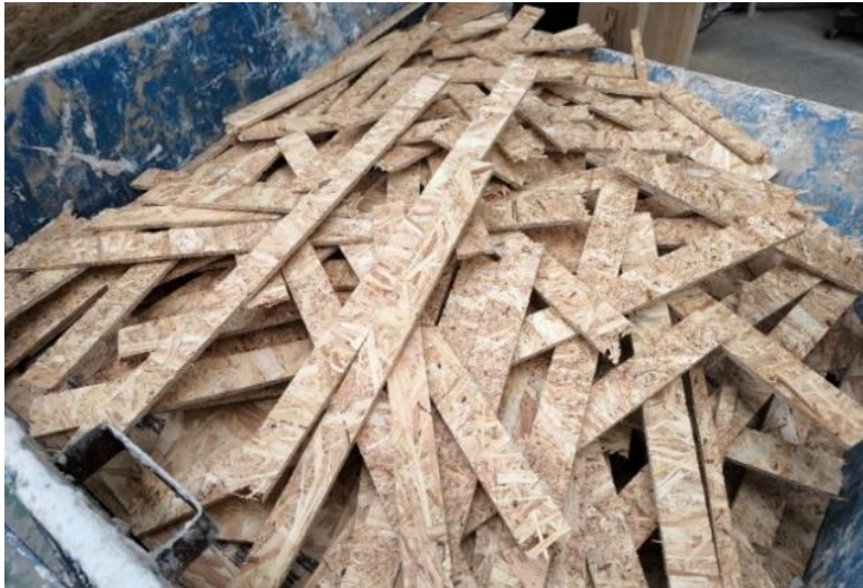
Figure 5.19: Length-side OSB offcuts
