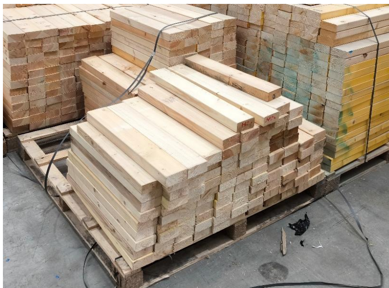
Figure 5.41: Excessive accumulation of 646 mm offcuts
