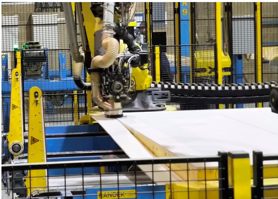
Figure 5.36: Width-side OSB offcut generation
