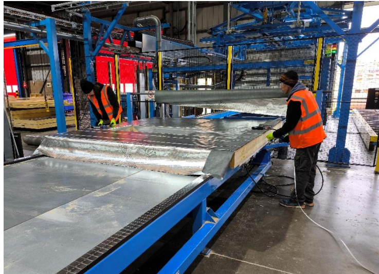
Figure 5.39: Fitting and cutting breather membrane
