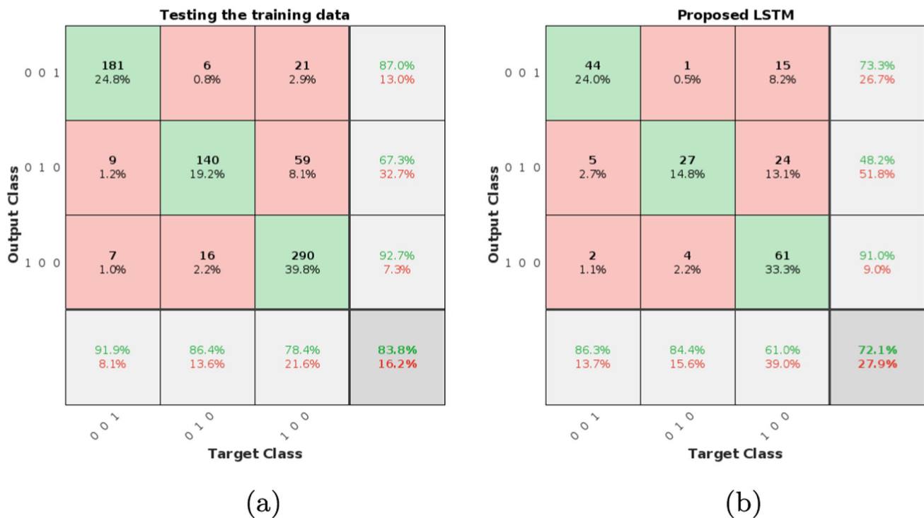
Fig. 14 Confusion matrix representing the performance of the Data-driven LSTM a) Training data accuracy. b) Testing data
