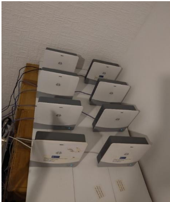
Figure 4. 6: Co-location test configuration using eight uHoo Aura sensors (left).
