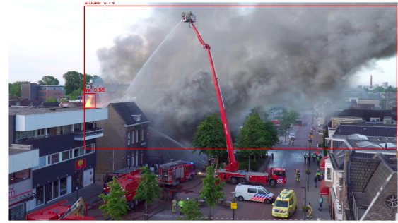
Fig. 6. YOLO11 “Flare Guard” output on a hazard scene showing detected smoke (0.74) and fire (0.55) regions. These confidence scores are interpreted as hazard severity indicators and are used to elevate environmental risk, triggering SORA’s escalation and emergency response policies in safety-critical scenarios.
