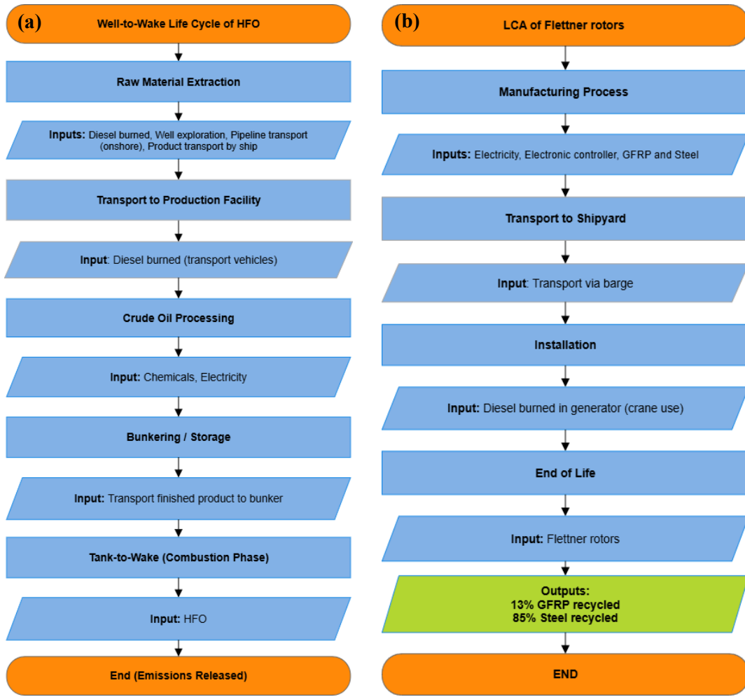
Figure 3. LCA methodology for (a) the well-to-wake ship emissions, and (b) for Flettner Rotor.
