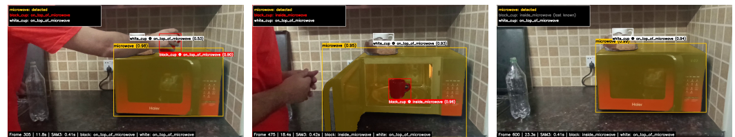
Figure 5. Perception under occlusion in the microwave task. (Left): the white cup, partially occluded on top of the microwave. (Middle): the black cup inside the open microwave. (Right): door closed and appliance running, with the black cup fully occluded and yielding no mask.
