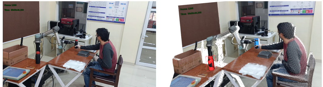
Figure 7. Zero-shot 6-DOF pose estimation from monocular RGB video. (Left): input frame. (Right): estimated poses rendered as textured mesh overlays on the scene point cloud, combining Any6D [34], Depth Anything 3 [35], SAM 3 [32], and a SAM 3D [36] reconstructed mesh.
