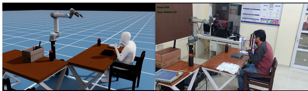
Figure 13. Side-by-side comparison of the Isaac Sim digital twin (left) and the real workspace (right).
