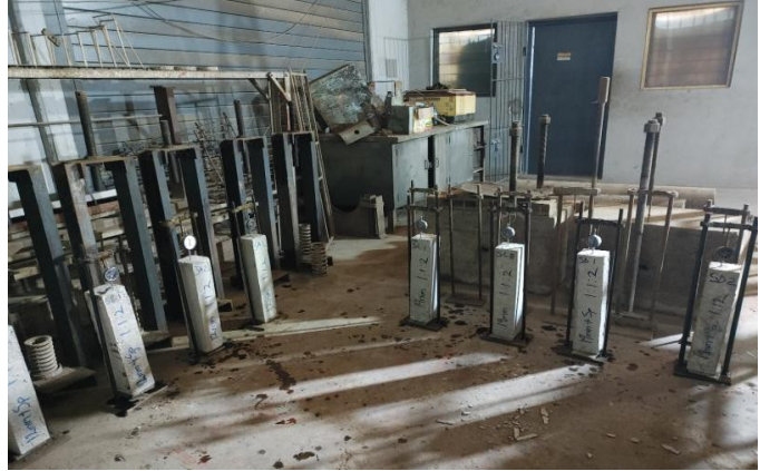
Fig. 4 Set up for drying shrinkage test
