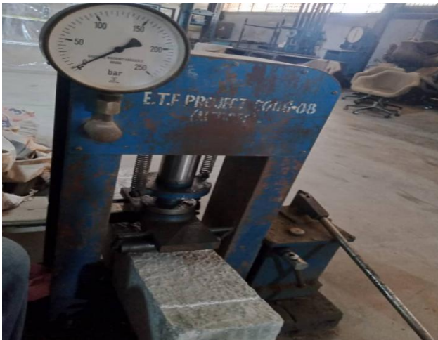
Fig. 2 Flexural strength test
