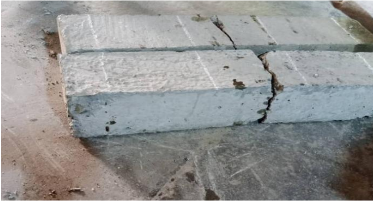
Fig. 7 Failure pattern of test samples
