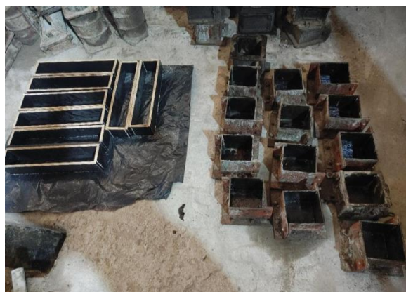
Fig. 1 Moulds for casting concrete cubes and short columns
