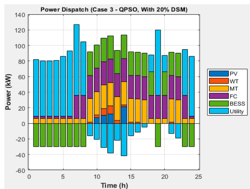
Figure 11. Schedule power profile of PV, WT, FC BESS, and Utility with 20% DSM.
